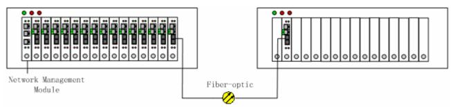
B. The both modules are installed in 16-slot 3U-high chassis, but only the host-site chassis is equipped with network management module. The remote-site module shall be set to "forced remote network management mode". That is to say, the 8<sup>th</sup> switch shall be turned to ON.
