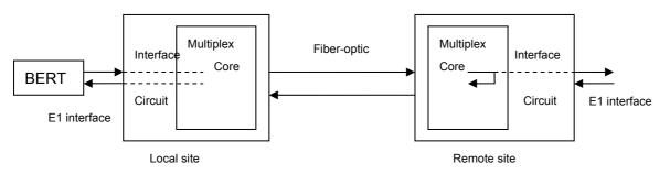
"E1 remote loop-back" setup at local Ethernet Multiplexer
